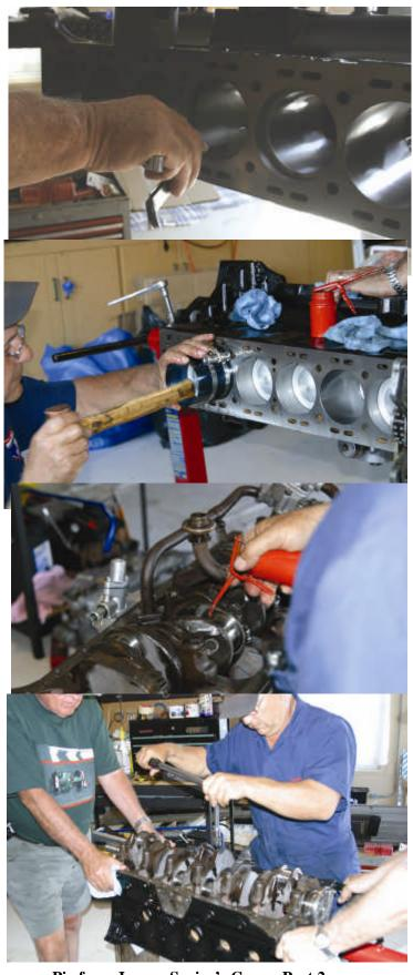
Pix from Jaguar Senior's Camp; Part 2 Measuring the ring gap; Inserting the pistons; Oiling the crank; Torqueing the crank
